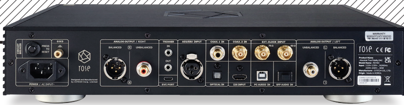
ABOVE: Digital inputs span optical (192kHz/DSD64 DoP), two coaxial and AES/EBU (384kHz/DSD128 DoP), HDMI/I 2 S (768kHz/DSD512), USB-B and SFP (768kHz/DSD512). Two clock ins are included, plus balanced (XLR) and single-ended (RCA) analogue outs
